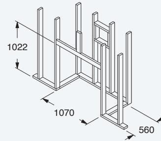
Dimensions above are in millimetres and for reference only. Refer to installation manual for detailed specifications on installing this product.
